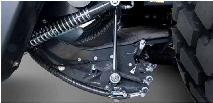
The 25-knife SuperCut chopping system features group selection giving a choice 6, 12, 13, 25 knives to match all conditions, all backed up with the security of a drop floor in case of blockage.
