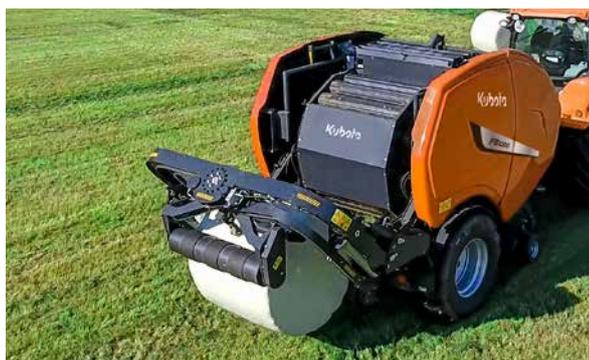
With the bale on the wrapper, it is then raised allowing the twin satellites to wrap the bale.
