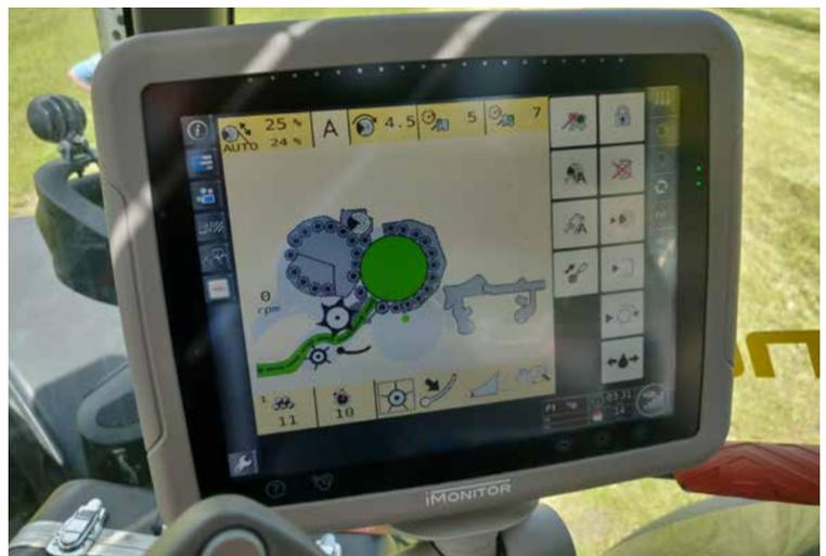
FB1000 is fully ISOBUS compatible as standard and can be operated on any ISOBUS equipped tractor without the need for an additional terminal.
